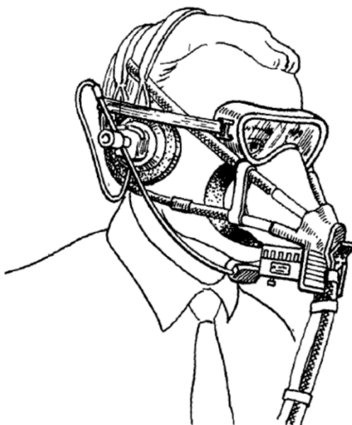
Fig.9 Oxygen equipment for crew members (KM-114M)
